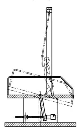
Figure 2 - Schematic drawing of the ramp method
